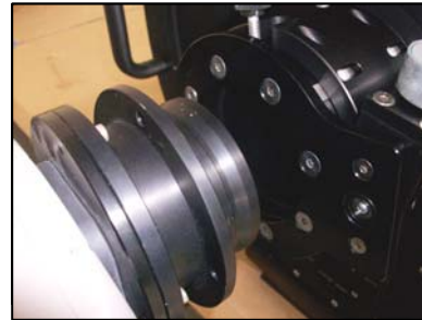
3 - Insert the 3.5" barrel of the 200166 Reducer into the 3.5" focuser securing with the two set screws on the focuser.
