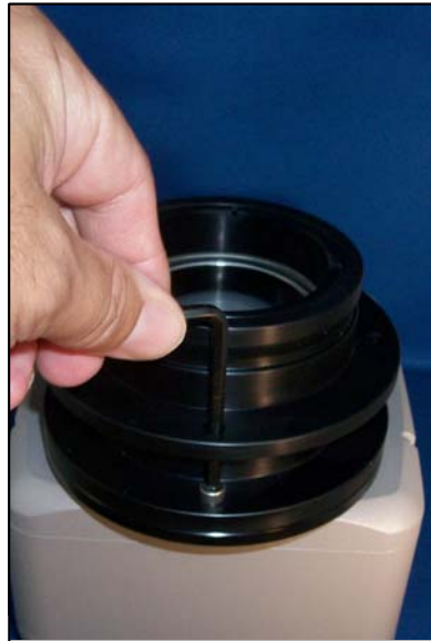
2 - Attach the 200166 Reducer to the SecureFit CCD Adapters using the four 10-32 SHC screws provided.
