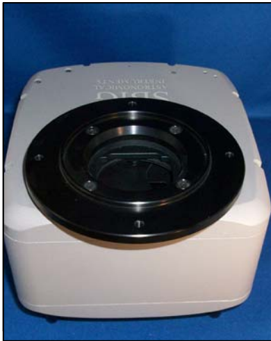
1 - Attach the 200362 (the SecureFit STL CCD Adapter) to the STL camera body.
